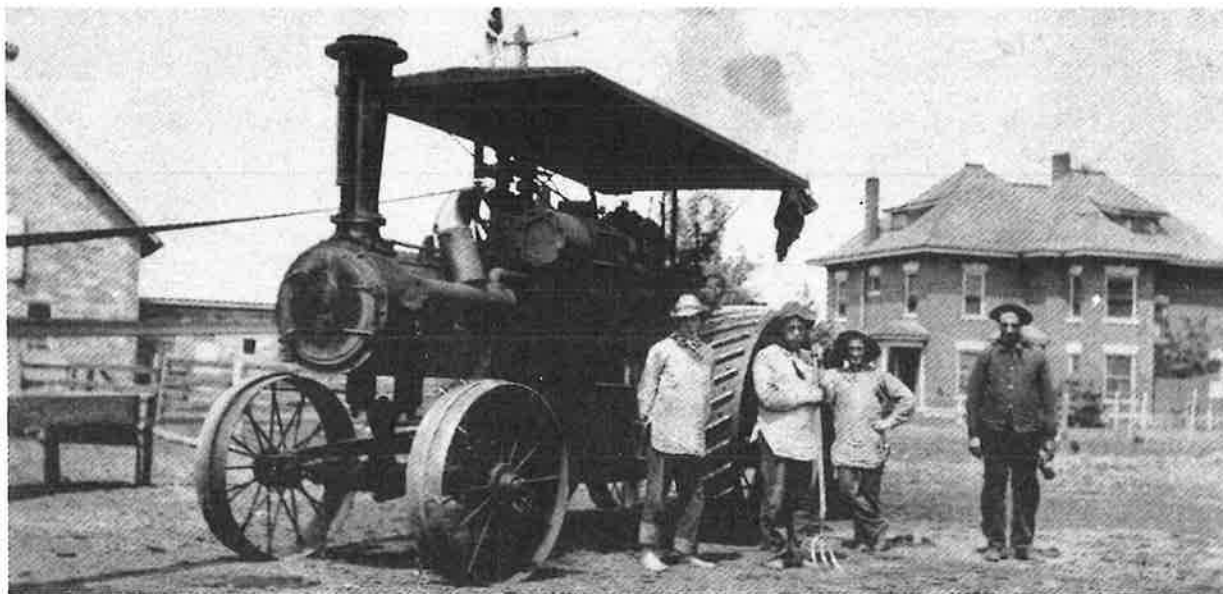
Steam engine used for threshing and power for saw mills. Picture taken at Matt Sexauer home on North Ash Street.
